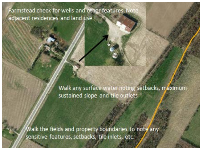
An example of dividing a site up into sections for the on-site assessment
